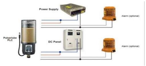
Above connection (brown + blue) method is for PNP type PLC lubricator.
